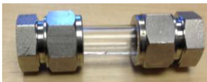
Figure 9. Test piece (TP) used for pilot-scale drying tests. The crack is visible as a white line towards the bottom of the sample.
